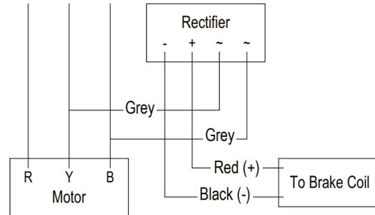
Brake coil is energized by DC side switching as shown in the diagram.
